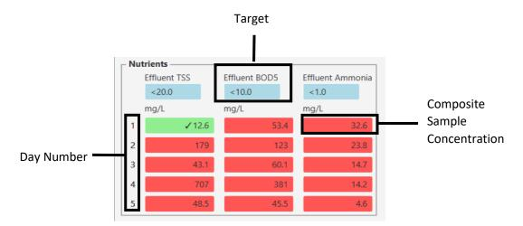
In order to score points, **all 5 composite samples must meet the target** (for one particular parameter, such as TSS). If the target is met for all 5 days, **75 points** are scored. For example, all 5 TSS composite samples must be below 20 mg/L in the example above, and since the samples on days 3,4 and 5 do not meet the target, zero points would be score for TSS.
