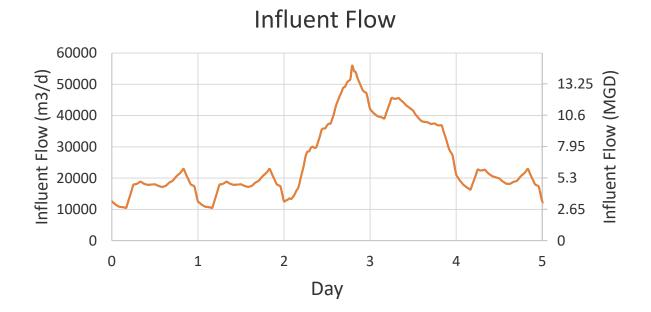
Note that a large wet weather event happens at the end of the 3<sup>rd</sup> day. The base wastewater influent concentrations are kept constant but are diluted with the stormwater flow. In this question, one secondary clarifier is out of service for maintenance purpose. The blower capacity is 2,450 ft<sup>3</sup>/min (100,000 m<sup>3</sup>/d).
